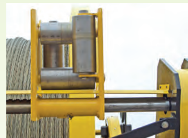
Automatic Hydraulic Level Wind
