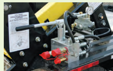
Hydraulic controls for complete control of the reel
