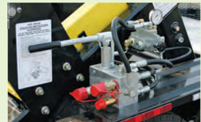
Hydraulic controls for complete control of the reel
