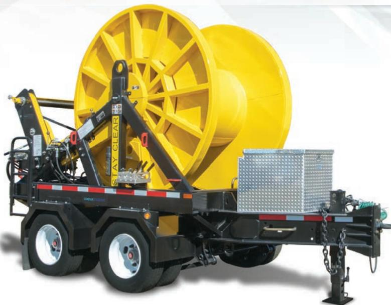
The Condux Tesmec **RW23 Hydraulic Reel Winder Trailer** is designed to work with the Condux Tesmec Pullers & Puller-Tensioners, and can be operated independently when powered by the 21011815 hydraulic power pack. It is equipped with automatic level wind and negative self-acting hydraulic brake. The RW23 can be equipped with the following: The Condux optional Fixed Steel reel, with 5/8, 11/16, 7/8 or 1¼ inch (16, 18, 22 or 31 mm) steel pulling rope of varying capacities.
