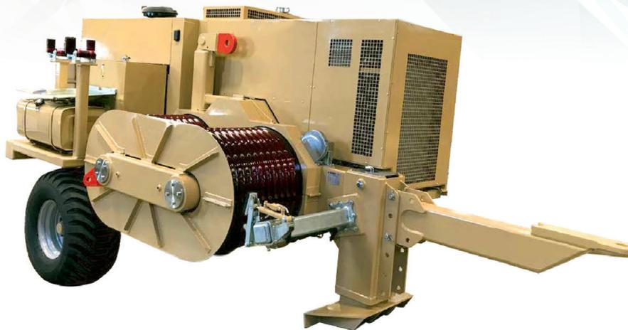
The **PL1950** offers 63,000 lbf (280 kN) of pulling force respectively and is designed for stringing **one rope** up to 1<sup>5</sup>/<sub>32</sub> inch (38 mm) in diameter.
