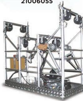
Aluminum alloy inspection trolleys allow two persons, in a standing position, to inspect two, three and four bundled conductor lines. The trolleys are equipped with spacers and insulators on top, along with stationary brakes and a meter counter.
