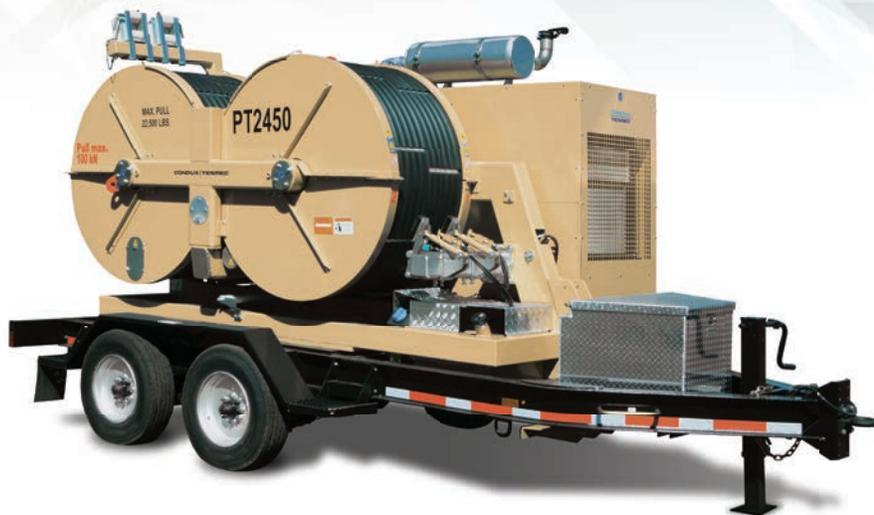
The **PT2450** features two pairs of independently controlled bull-wheels, offering 2 x 11,240 lbf (50 kN) or 1 x 22,480 lbf (100 kN) of tensioning capacity for stringing one or two bundled conductors. The bull-wheel grooves on the PT2450 are made from high resistance interchangeable nylon sectors. The PT2450 features a new digital interface with 7-inch color display, wireless remote, integrated pull/speed recorder and remote diagnostics.
