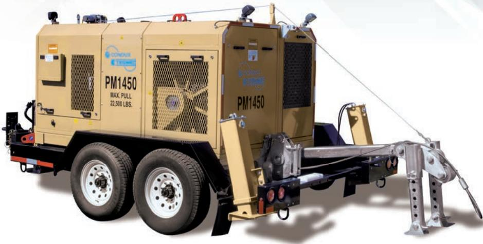
The **PM1450** offers 22,500 lbf (100 kN) of pulling force and is designed for stringing **one rope** up to 5/8 inch (16 mm) in diameter. The bull-wheel grooves on the PM1450 are made from heat treated steel.
