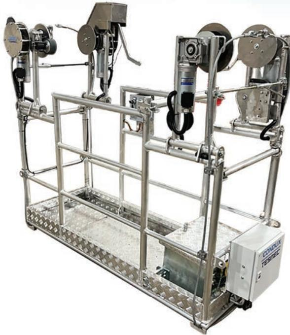
The Condux Tesmec **CRT840 Inspection Trolley** is suitable for work on two, or three bundled conductors. The trolley is powered by four electric motors and an on-board battery. The unit provides easy lever and joystick control for speed, direction and brakes.
