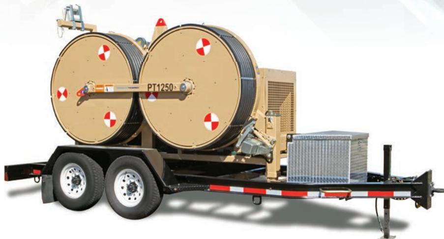
The **PT1250** offers 11,240 lbf (50 kN) of pulling or tensioning capacity and is designed for stringing one rope or one conductor. The bull-wheel grooves on the PT1250 are made from high resistance interchangeable nylon sectors. The PT1250 features a new digital interface with 7-inch color display, wireless remote, integrated pull/speed recorder and remote diagnostics.
