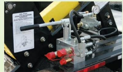
Hydraulic controls for complete control of the reel
