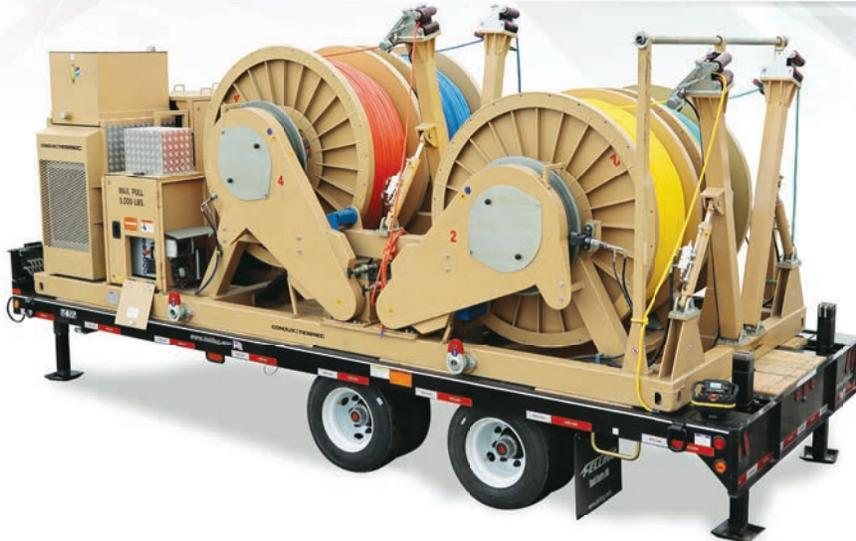
The **PD4500** 4-drum puller tensioner offers the ability to string new conductor, as well as perform reconductoring operations, over than the typical stringing of pilot wires.
