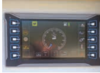
NEW DIGITAL HMI The 7-inch color display indicates machine working parameters, maintenance records and has integrated pull and speed recorder.
